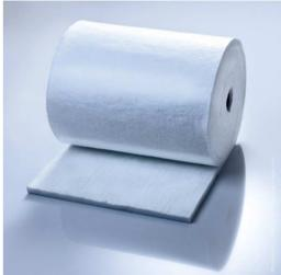
**ITM-Fibermax®** blankets are high temperature, lightweight and flexible products manufactured from polycrystalline mullite/alumina wool (PCW) that can be exposed to temperatures up to 1600 °C (2912 °F).
